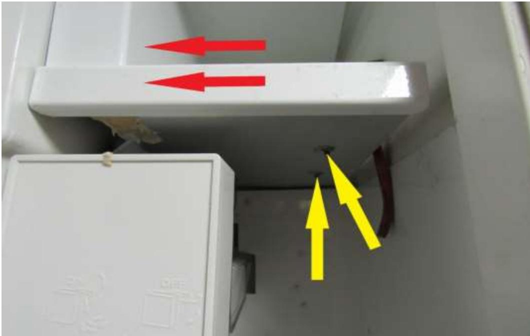
Now insert the 2 bolts to hold side plate, these can be hard to get lined up as you can't see in there, if you cannot get them in they don't have to be there as this plate is over against the cooling unit and held there by the bottom pc.
