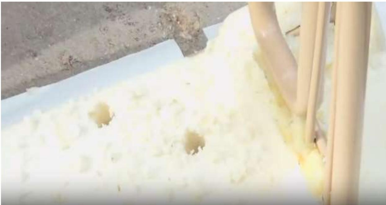
While it's still on its back apply the thermal mastic (included) place a small bead on the freezer tubes only where shown for now. **Red lines**
