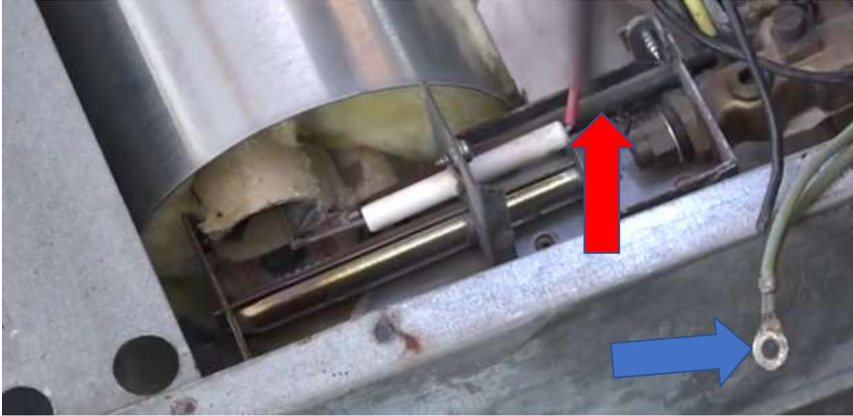
Plug the wire harness back in again (RA) and the heating element wires (YA) put board cover back on
