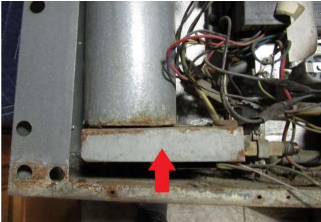
Remove the three burner mounting screws (RA).
