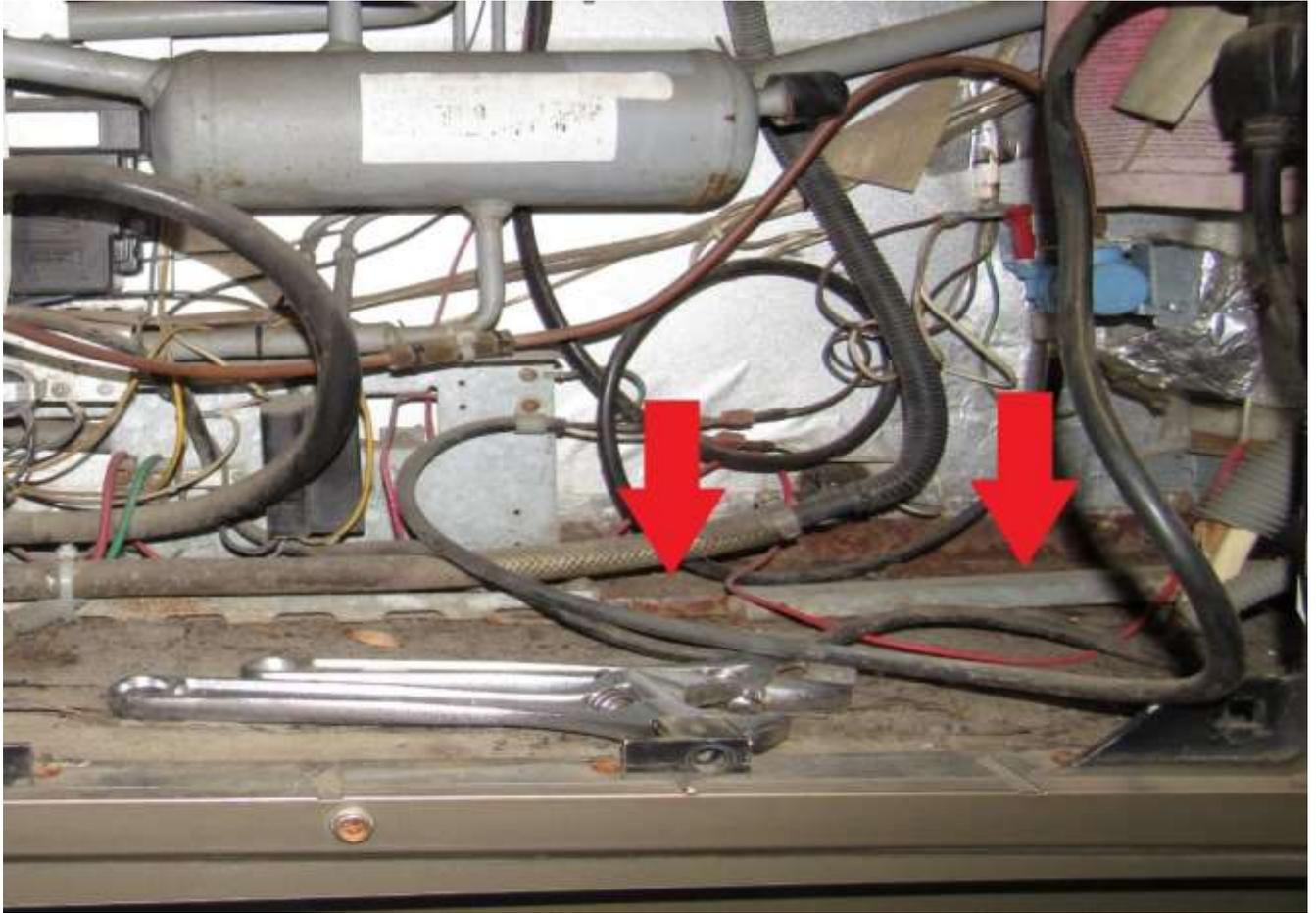
Remove top mounting screws (**RA**). It's a good idea to place all loose screws in a bin as you will need these later.
