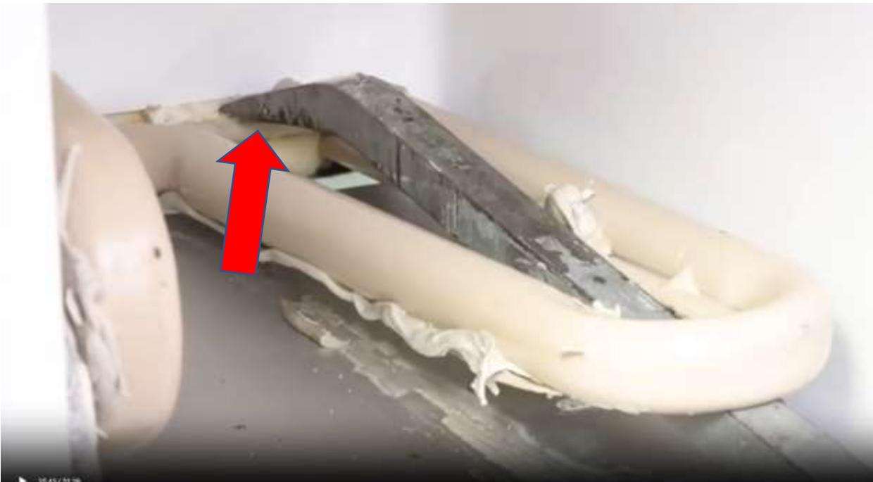
Line up the secondary system mounting holes in the center to our cooling unit plate holes, tube might have to be pushed back, up or down to get it there (BA) use original screws to fasten the 2 together.
