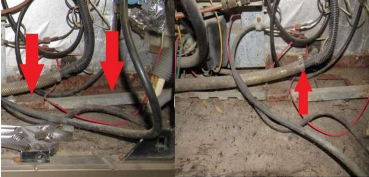
Reinstall your gas line, make sure its tight and after the gas has been turned on use soap and check for leaks on all gas joints. (RA) hook your 12V DC back up to the power block as before, make sure to put the positive back to where it was before. This is where you connect the interior fin fan and rear vent fan to. (YA)
