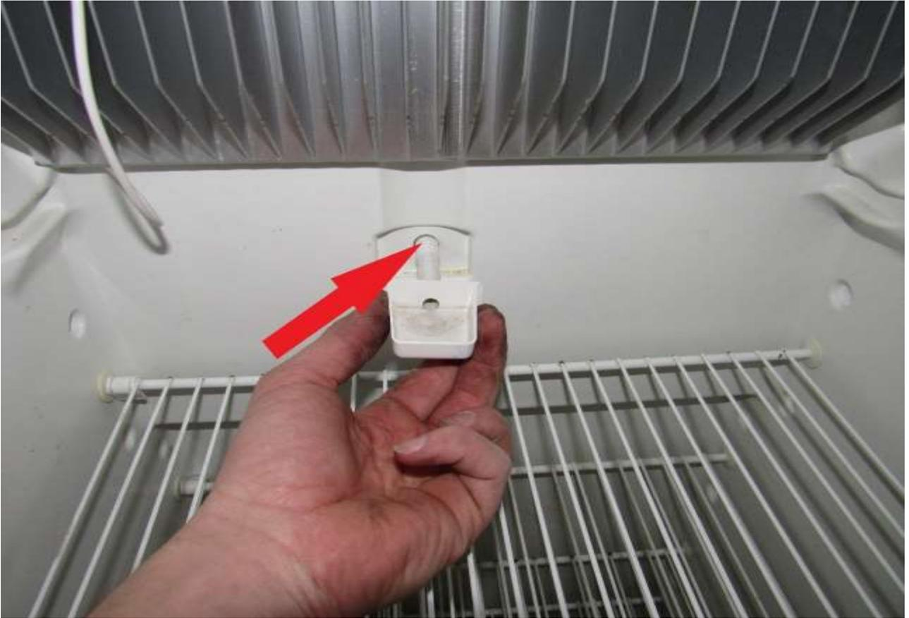
Have someone connect the defrost hose on the outside. You might need to enlarge the hole in the foam a tad to let the hose slide in over the spigot
