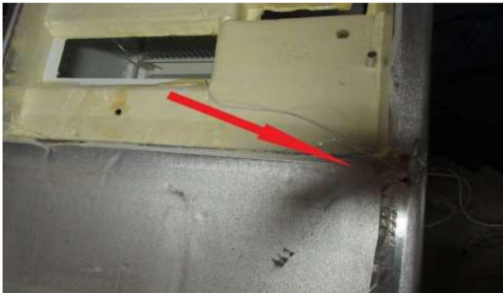
If you are using your old heating elements off your old unit lay old unit on its face and open the heater flapper by squeezing the boiler stack and opening the flapper. **(RA)** if you are using new heaters then skip this step
