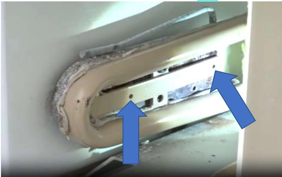
When your done in the front make sure the fin in the back is close to level to the box, it does not have to be perfect but only close. You may need to remove the 2 rear mounting screws if it needs to be pushed or pulled into place. Pushing the unit to the side will not put extra pressure on the tubing, remember these units are made with thick steel tubing.
