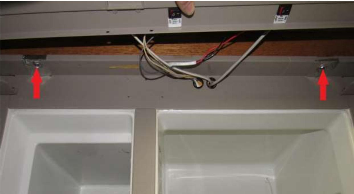
Fasten the screws that hold the top control panel into place (RA).
