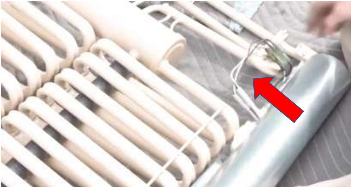
Now lay the unit on its back and if you are reinstalling your icemaker then the holes for the water spigot and icemaker wires will have to be predrilled in the foam. Take measurements off your old unit and use these as a guide to drill new  $\frac{3}{4}$ " holes onto the new, when drilling be careful to not hit a steel tube.
