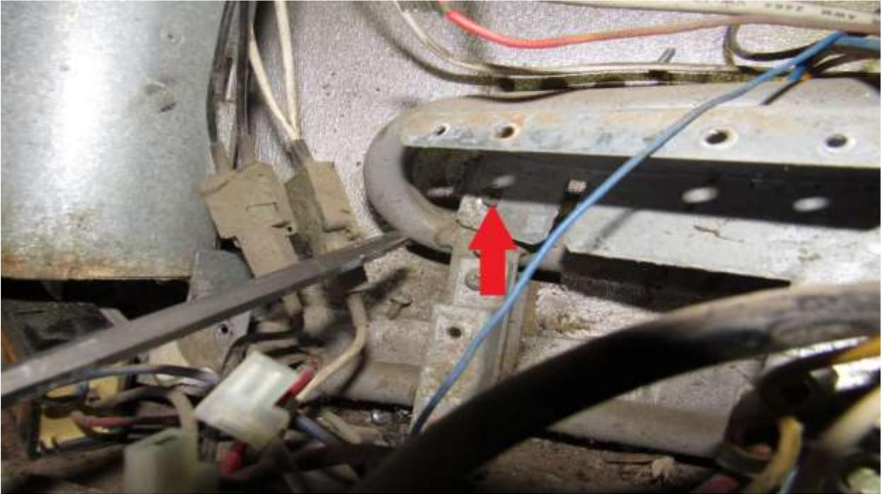
Remove these two mounting screws (RA).
