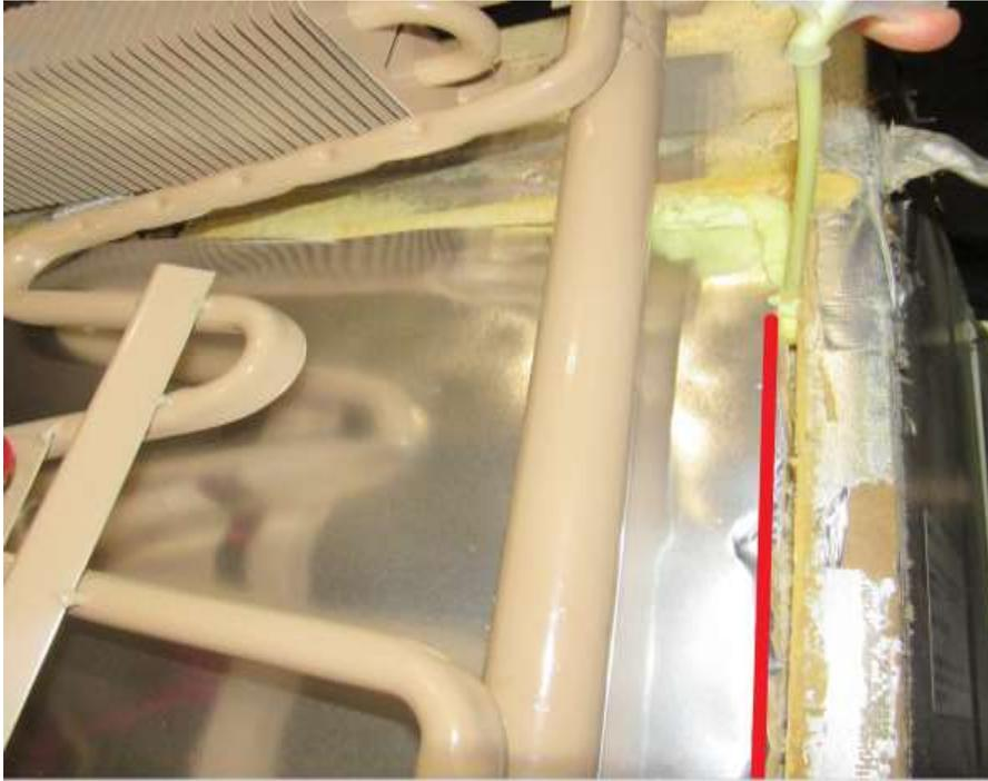
Make sure all 4 sides are completely sealed, add foam to the defrost hose
