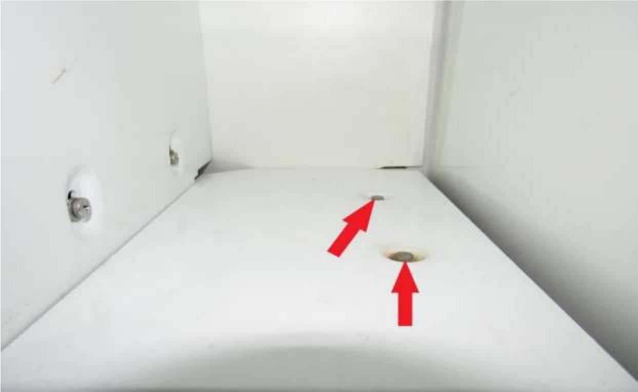
Remove the six mounting screws on side plate (RA). Remove the plastic piece (YA) and lay it aside for later.
