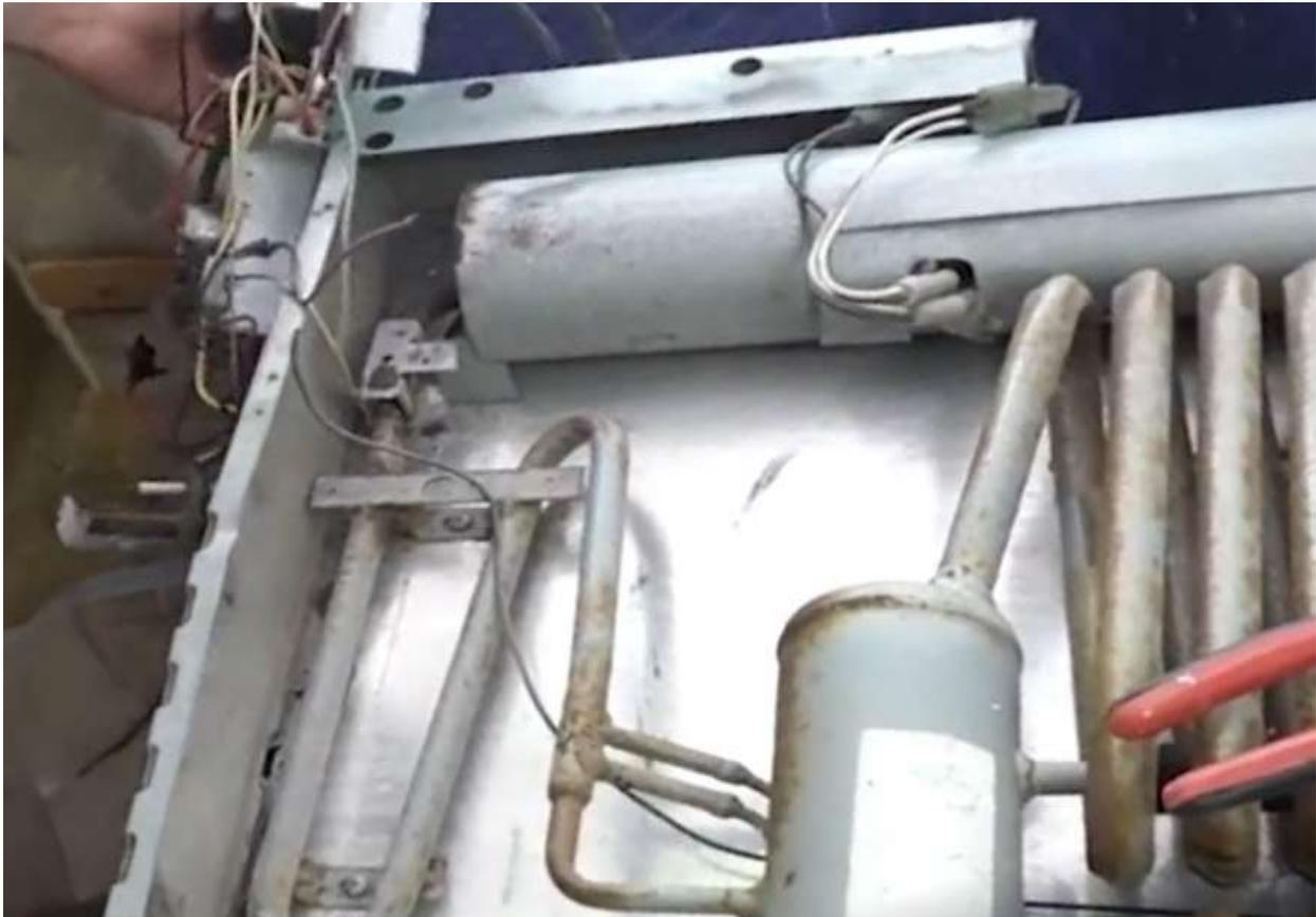
Lift the bottom of the unit up and remove the main ground wire (RA).
