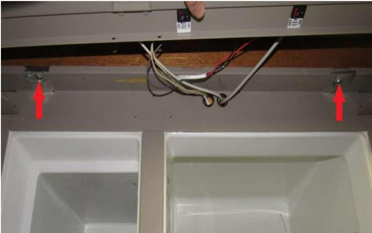
Secure the top control panel again with the two screws to hold in place (RA).
