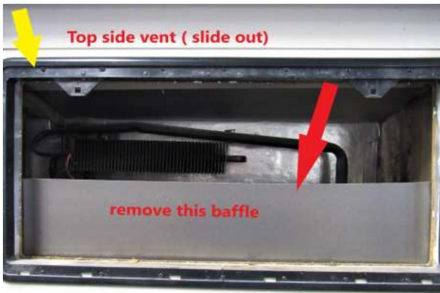
You will then be required to add a slideout fan to your top side vent to force the hot air out that's being pushed up from the fans below the vent, **(this is required on all slide out models to be covered in our warranty)**
