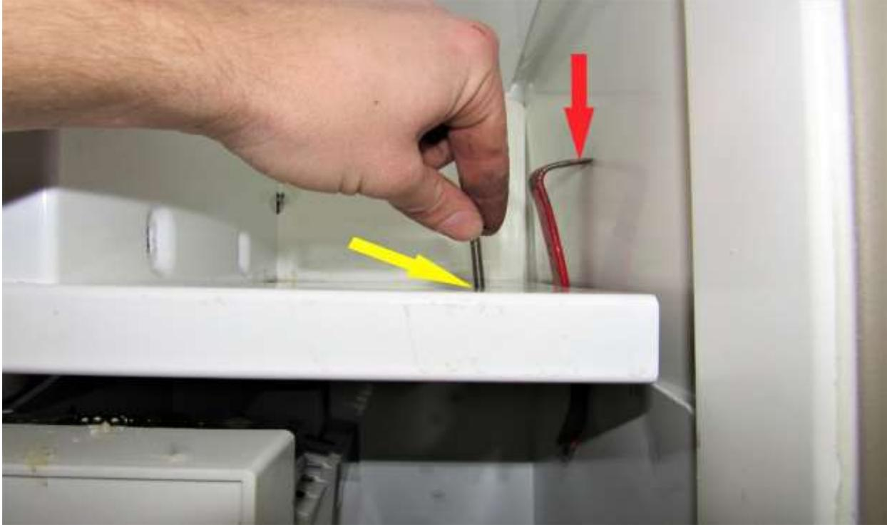
Thread the nuts onto the bolts (YA). using the pry bar apply enough pressure to shift the plates left as far as they go (RA). Then make nuts tight
