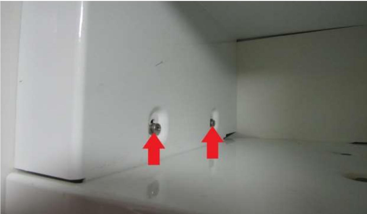
Remove the two mounting bolts on bottom plate (5/16 socket) (RA).
