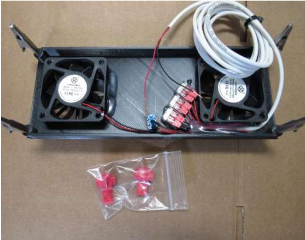
We Highly recommend adding a interior fin fan to the fridge area, skip this step if you're not adding the fan. Insert the fin fan into the fridge box through the fin opening (RA) push the defrost cup spigot into the box so it does not break off when new unit is installed (YA)
