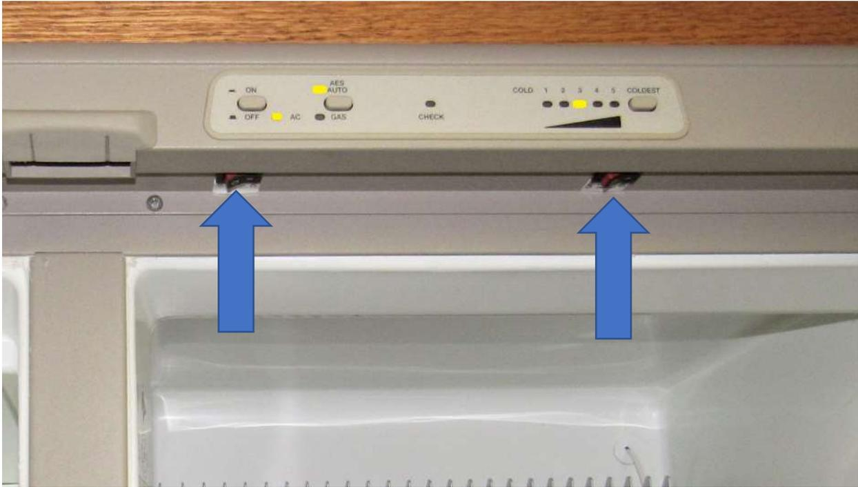
If you have a amp clamp the total amps between the 2 heaters should be 3.6A to 3.8A. After its been running for ½ to 1 hr you need to make sure you here the rear vent fans turn on. Which can be heard either thru the front fridge door or thru the rear side vent.
