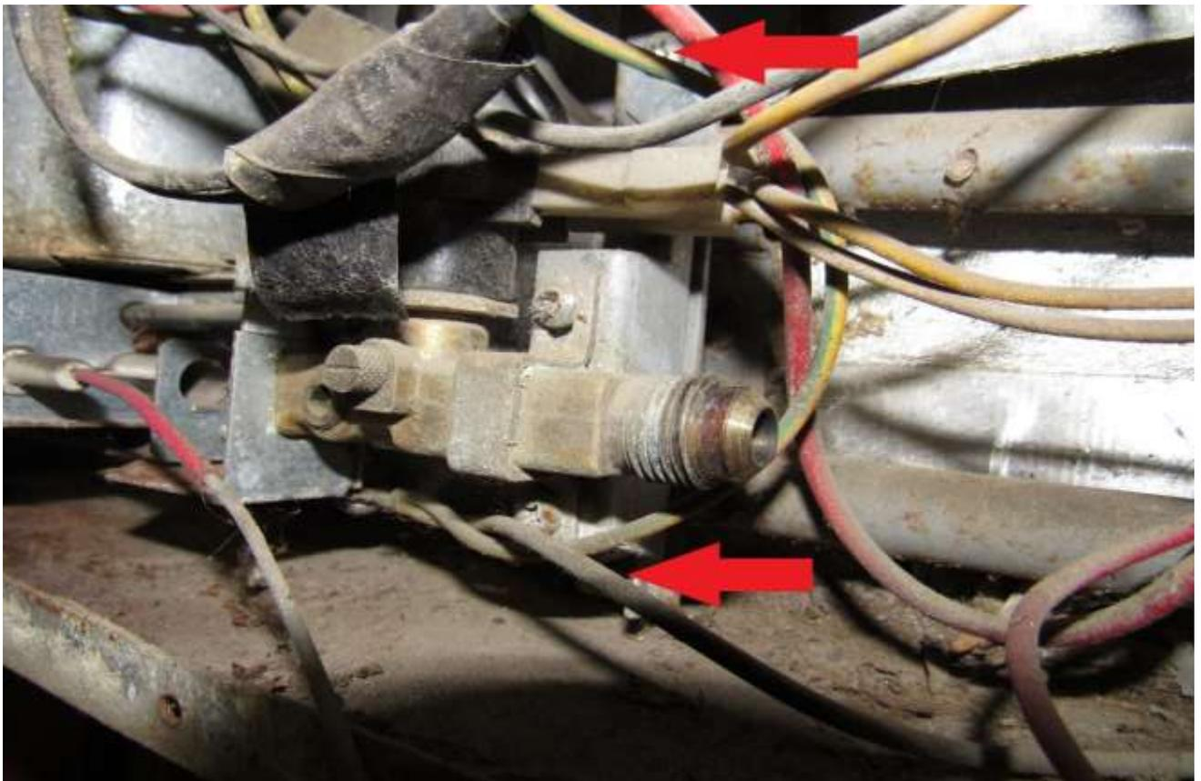
Remove board mounting screw (RA). This could vary some as Board styles vary.
