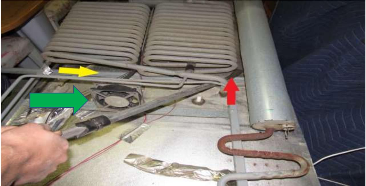
Remove the small angle plate where the LP burner was located (RA). Clean bottom of unit with a vacuum getting rid of all dust and rust.
