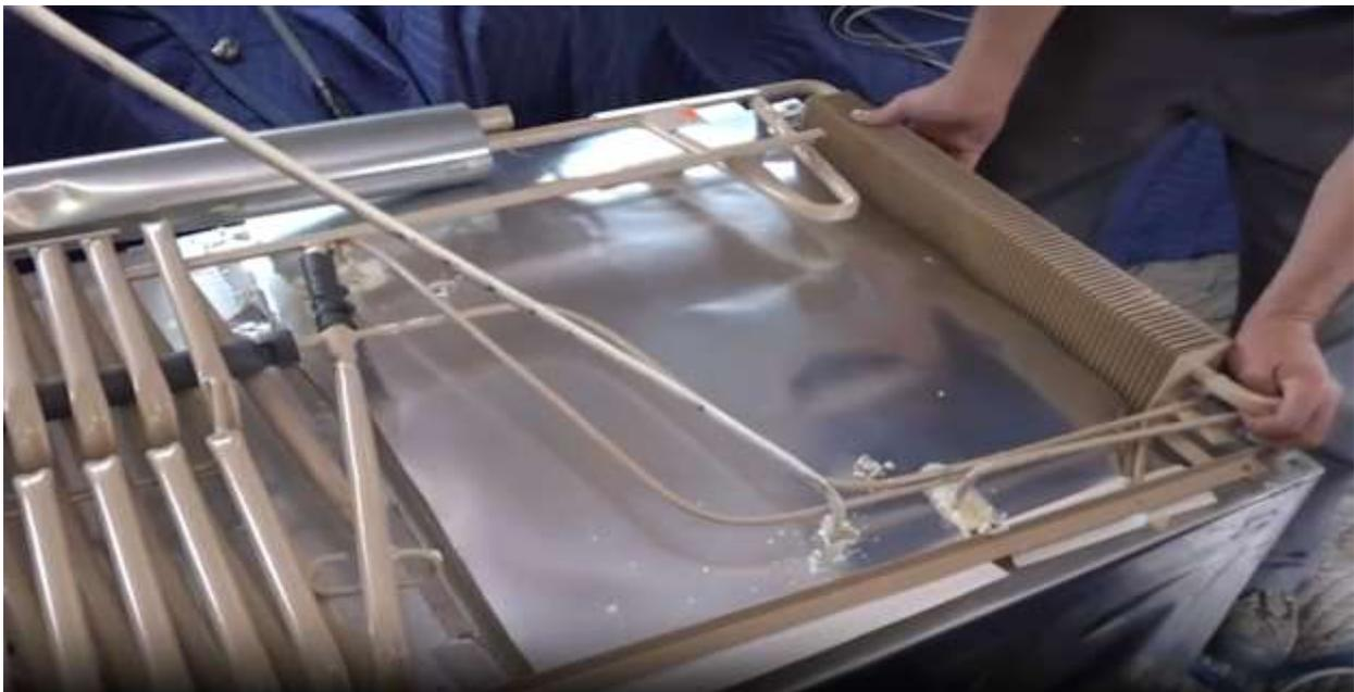
If your new cooling unit does not slide in level with the box then this is nothing to be alarmed about as once the fridge fin is installed this will pull in tighter.
