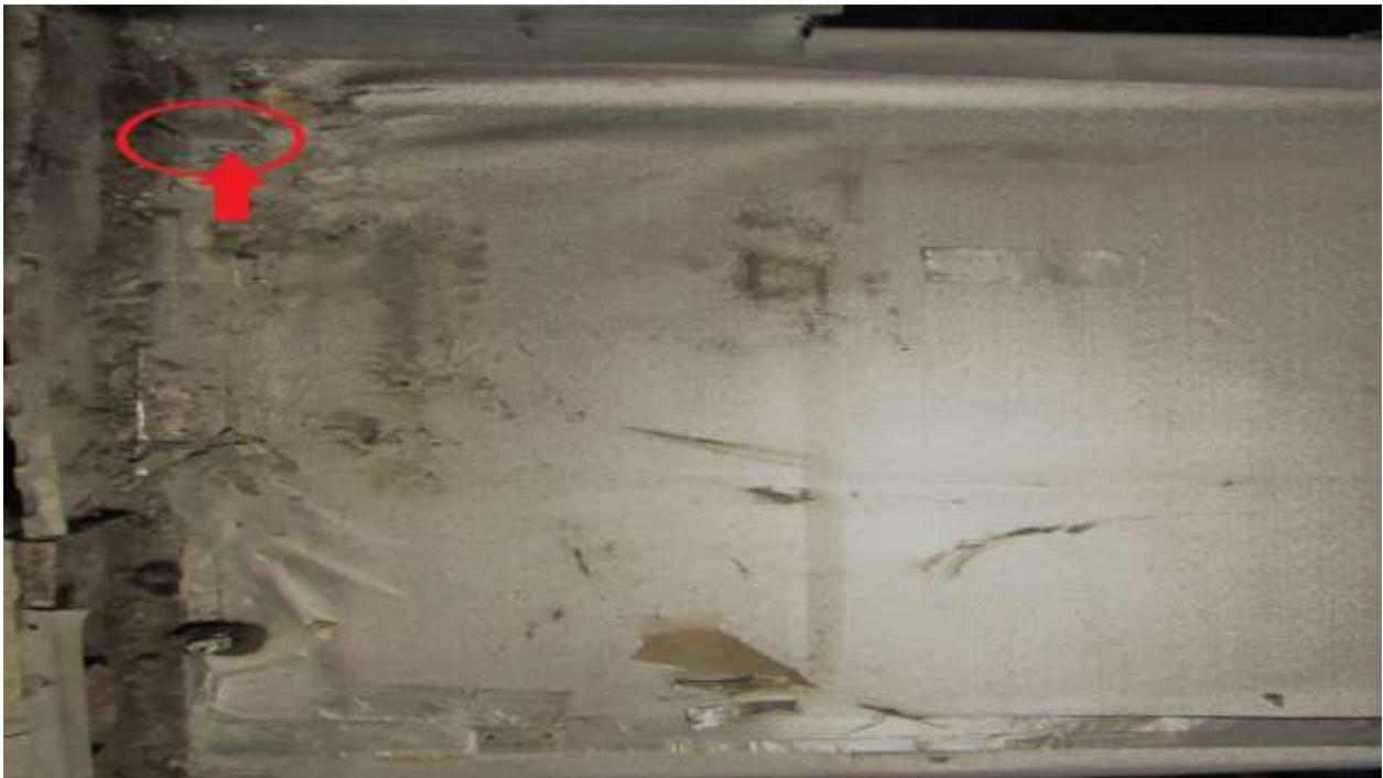
Clean foam and debris on all four sides, make sure all excess foam is removed, check corners as well (RA). Use vacuum if needed to clean box
