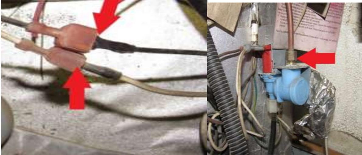
Insert the icemaker water spigot again into the back of the unit making sure its inline with the icemaker, add foam to seal around the spigot & wire
