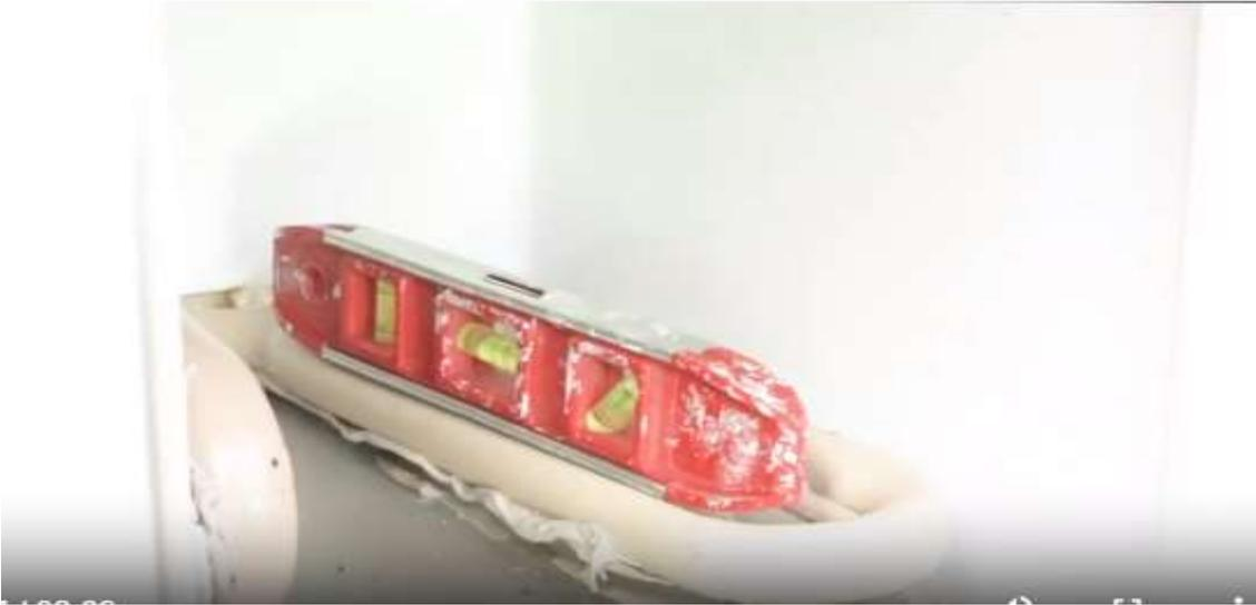
If your box has been leveled like shown above then this tube will need to be perfect level as well. If its not level with your box then take a pry bar and use the small brace welded across the back (RA) as a hook to go either up or down as needed. The one we show here needed to go up so the bar is slid between tube and icemaker plate.
