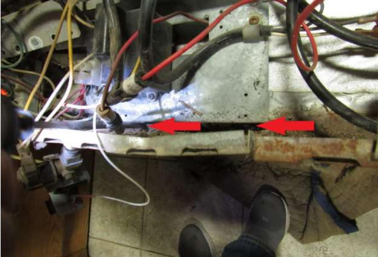
Remove the top plate mounting screw (RA).
