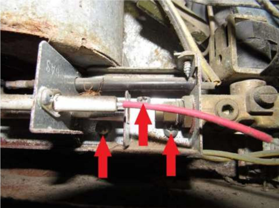
Remove two LP bracket mounting screws (RA).
