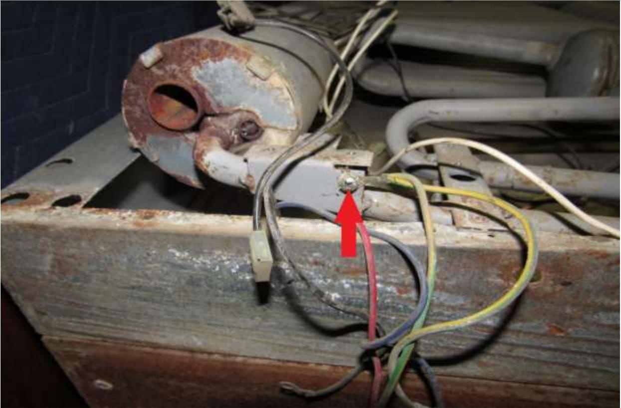
Remove the defrost tube (RA).
