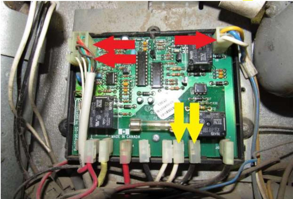
Disconnect red wire (RA) and cut the black ground wire (YA). This is your interior light wire, so this will have to be spliced back together later
