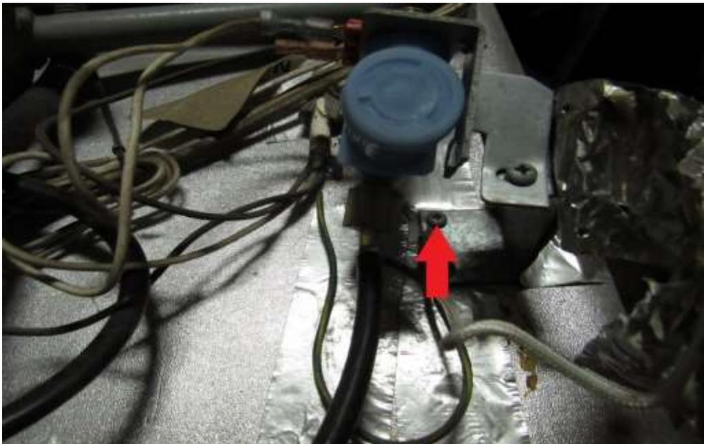
Reattach the 120V wires for ice maker cord (RA). Reattach water line
