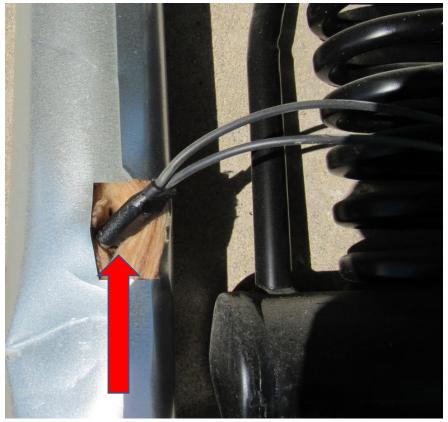
lay the new unit on its back. Open the heater cover and push the insulation back so the heating element sockets are exposed, and slide the heating element into the socket. It does not matter which socket you choose. Make sure it's pushed all the way down to the stop point on the heating element. Push insulation back over the heaters and install the cover and tuck the heater wires out of the way for now. 1 extra socket is available should it be needed later
