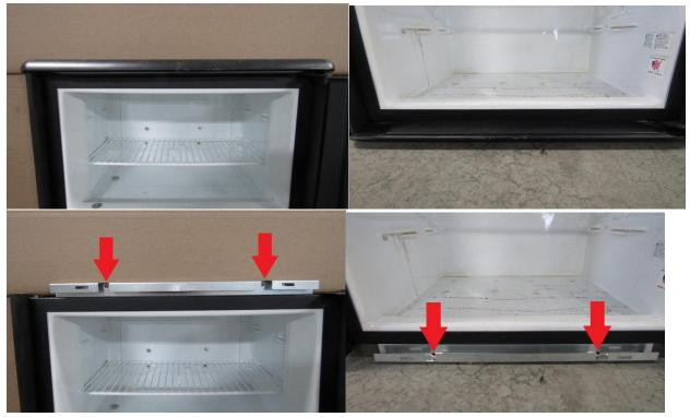
Take a 5/16" hex bit and cordless impact driver and proceed to loosen all the screws (RA) in the freezer and the refrigerator. Refrig fins will drop down so unclip thermistor and lay to the side, remove fins and set to the side for now. Removing your freezer shelve or top fridge shelve is optional.
