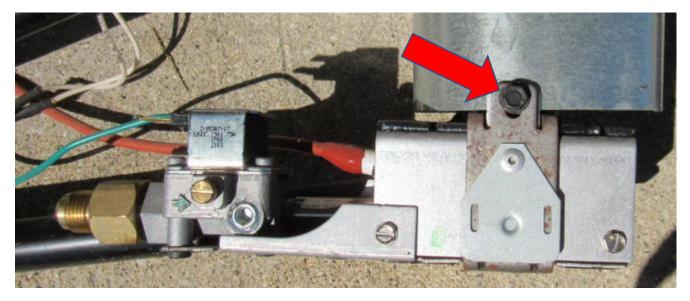
if you have purchased a new heating element with the new unit skip this step, if you are using the original heater unsnap the heater cover and slide heater up out of the heater socket. (RA)
