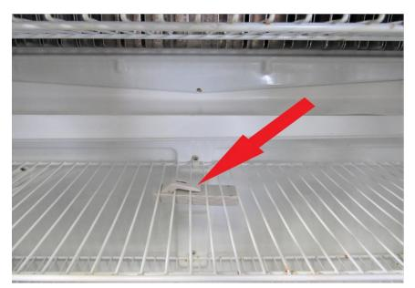
The same applies the with freezer. Clip the sensor underneath the shelf, centered from side to side, but have this one more towards the back of the freezer.
