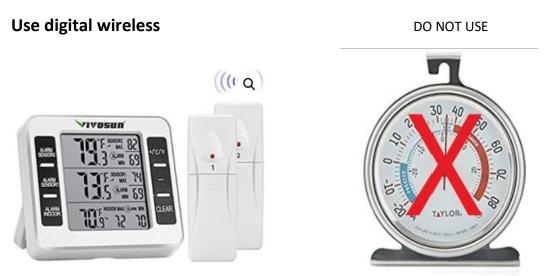
Clip the sensor for the fridge on the bottom side of the first shelf beneath the fin, place it so the sensor is centered, front to back and side to side (RA), if its clipped underneath it will be out of the way and shouldn't interfere with storage.
