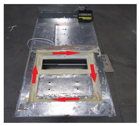
Clean off the old thermal mastic (RA) from the freezer section. A large blade putty knife or scraper works well.
