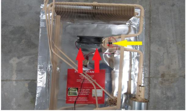
Take unit off the back of your refrigerator by lifting straight up and out. Clean off any residual foam or thermal sealant around the edges (RA).
