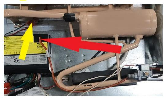
Take the heating element wires (RA) loose from the board. Leave the 120V plug (YA) on the board.
