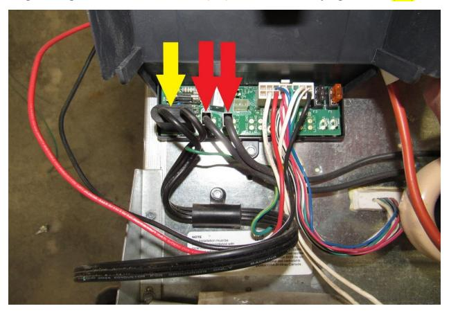
Plug heating element into the board (RA) make sure 120V plug is intact (YA)
