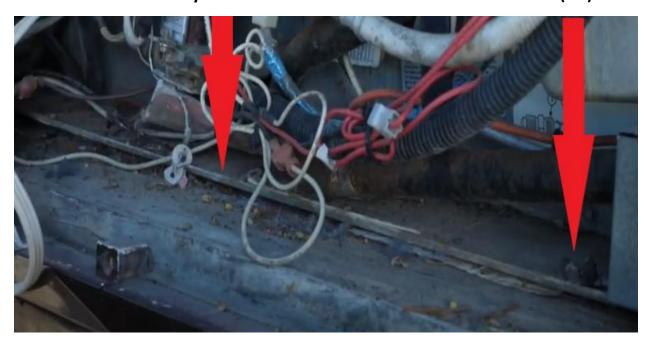
On Winnabago coachs you will have 4 bolts lagged to a steel side plate, 2 on each side of the fridge, also the top roof vent cap needs to be removed and 2 to 4 philips screws need to be loosend from the top of the fridge.
