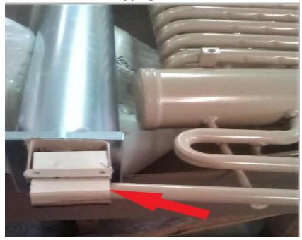
On the new unit, install the burner assembly first (RA) using the original screw. Followed by the igniter (YA) also using the original screw.
