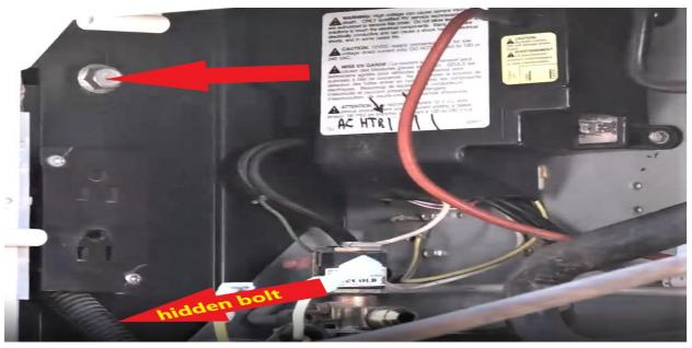
Going inside, remove the black trim buttons and remove the mounting screws
