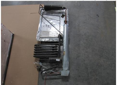
Clean off the old thermal mastic (RA) from the freezer section and the fin section. A large blade putty knife or scraper works well.
