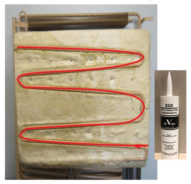
Now lay unit into box being careful so as not to scrape off any thermal mastic, feed icemaker lines up thru the new holes again, thermistor wire feeds out thru the side between unit and box. (RA)
