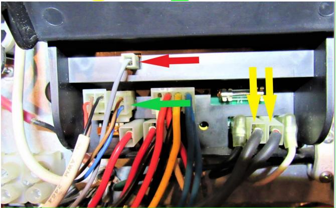
This relay should stay intact like it was originally, (YA) if you did remove wires for this then they need to be returned to the same spades as before. This might not resemble yours as these vary with the number of wires to this relay from fridge to fridge. Depending if a icemaker or water dispenser is on the fridge.
