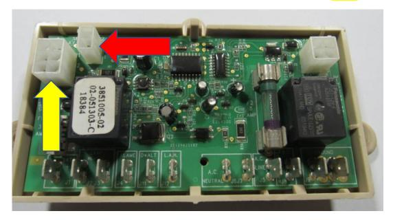
This is the more common board: Take a screwdriver and gently pry out both sides of the board to release the cover (RA).
