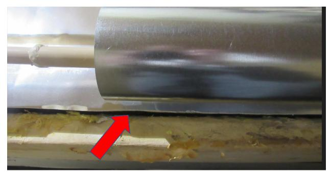
In some areas it might seem to be tight against the box, and in this area cut back enough foam on a angle to create a small gap off the unit so you can get your foam straw in to fill the void further down. We cannot stress enough on this step because if even a small 2" gap is left open it will not cool in the fridge like it should.
