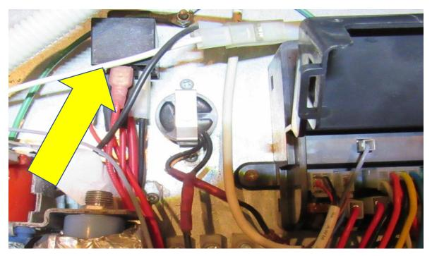
This is the time to rewire your icemaker back to how it was originally, and push your defrost hose onto the spigot (RA) You are now ready zip tie all your wires, tuck 120V cord to the side and clean everything up to get ready to slide the fridge back into the cavity
