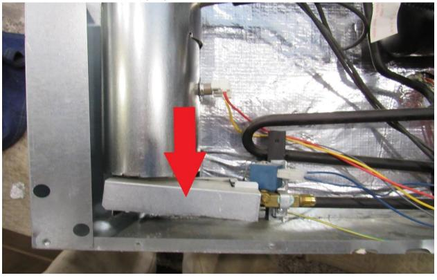
Remove the burner cover (RA).
