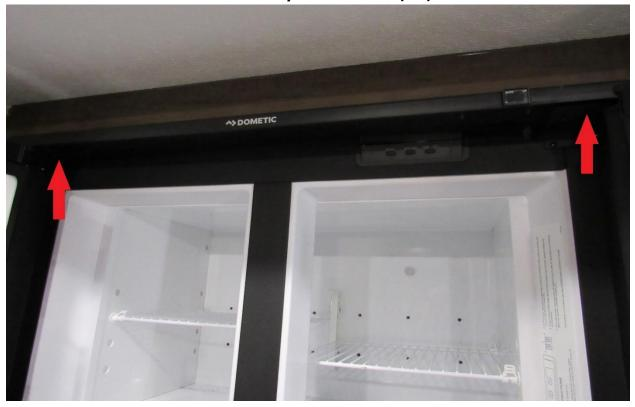
Remove the screws from the front eyebrow board (RA).
