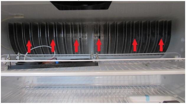
Install all the screws into the refrigerator fin (RA).
