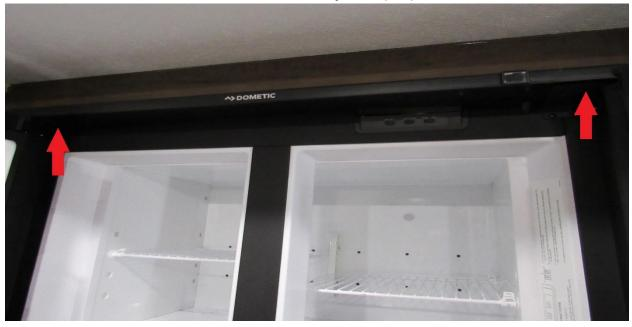
Remove the screws from the front control panel (RA).
