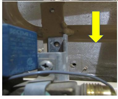
Unsnap Heater flapper and separate the insulation till you find the 2 heater sockets (YA)
