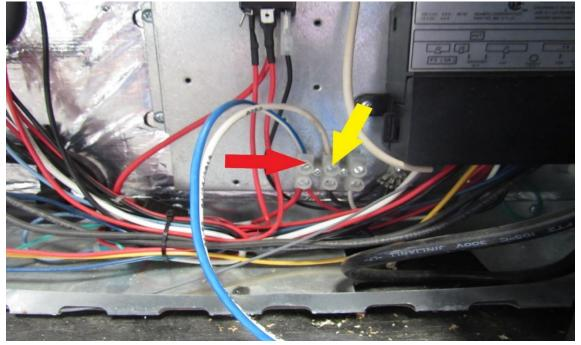
Cap off the 12v positive wire as it is not insulated (RA). These can be stuck to the side out of the way for now
