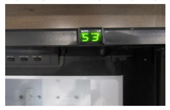
Now plug your 120V plug back into the wall outlet and make sure you have 120V AC power to this outlet. LP burner should now shut down and board should switch to AC. If you have a amp clamp the total amps on the heaters should be 3.6A to 3.8A. After its been running for ½ to 1 hr you need to make sure you here the rear vent fans turn on. Which can be heard either thru the front fridge door or thru the rear side vent
