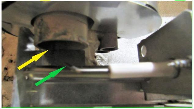
Refasten Lp Burner back onto the burner brackets, (YA) Make sure to use the short screws back where they were, do not use the self-drilling screws where the short screws were. Otherwise, you will puncture the tube beneath.
