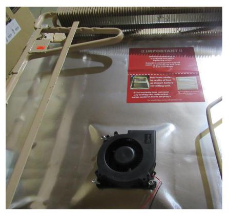
Make sure fan is pointing up and use the screws supplied with the fan kit
