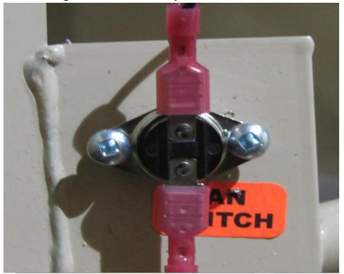
The 12V DC supply wire for the fan needs to be attached to your coach 12V DC wire later.
