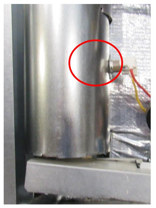
Most times Your fridge has 2 or more vent fans on the center of the unit blowing air up, these can be reattached same as they were on the old unit, make sure they are pointed up and the fan switch needs to be located on the plate marked "fan switch" shown later. Or if you bought our recommended vent fan kit it gets mounted to the back of the unit marked "Fan Backer" this has a thin sheet metal backer to hold the fan into place.
