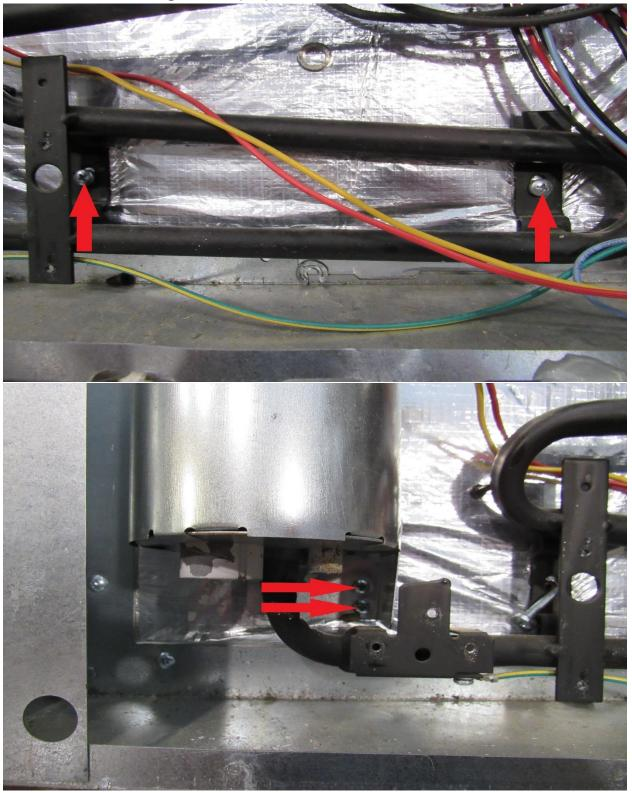
Remove the mounting screws (RA).
