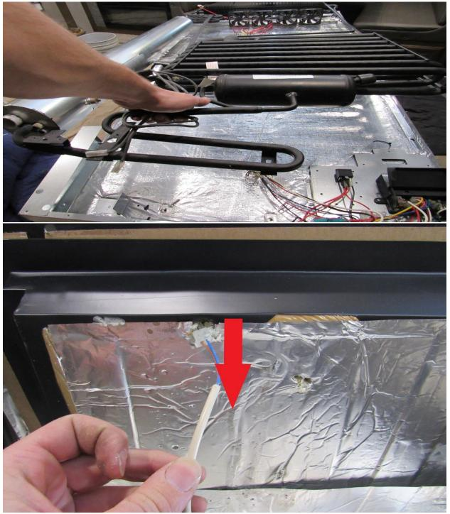
Clean all four sides (RA) and also clean any foam or thermal mastic off of the aluminum plates (YA).
