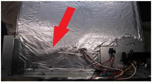
Clean and vacuum and debris on the bottom (RA).
