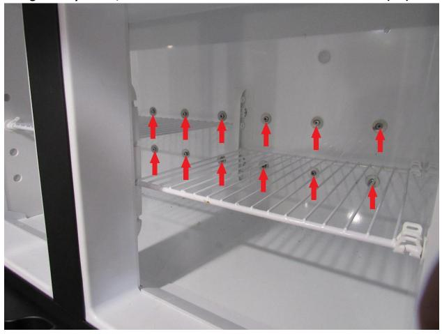
Going inside your RV, remove the freezer screws in the freezer section (RA).
