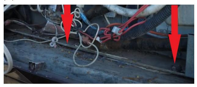
On Winnabago coachs you will have 4- 9/16" bolts lagged to a steel side plate, 2 on each side of the fridge, also the top roof vent cap needs to be removed and 2 to 4 philips screws need to be loosend from the top of the fridge.
