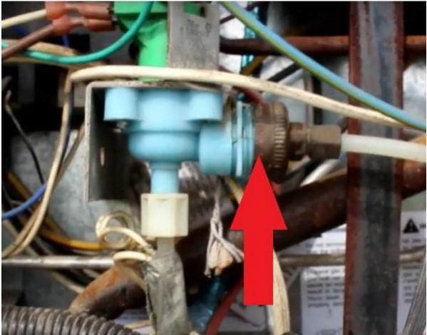
Using 2 wrenches remove the LP line (RA) off of the LP solenoid valve. Make sure LP gas is turned off.
