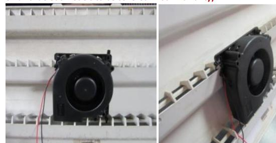
The eyelet can be screwed at any ground, connect female + to the fan switch wire, so it comes on when the lower fans come on
