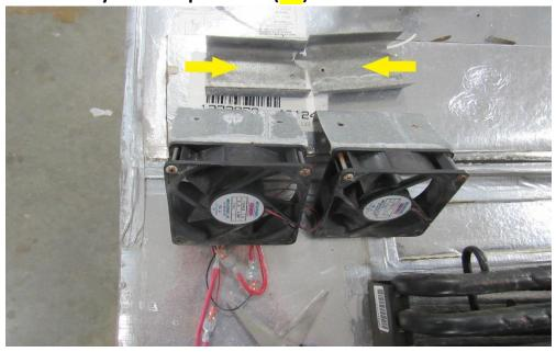
If you are replacing your ventilation fans, which we recommend, now is the time to do so. Start by removing the 4 screws (RA). Assemble the new fans in the same orientation as the old fans. Set the fans aside for now.
