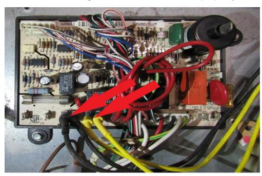
Remove the 4 heating element wires from board (RA). 2 yellow/2 black
