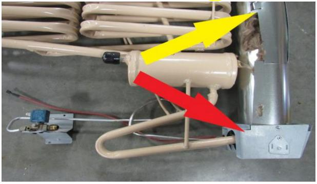
Push the insulation back so the heating element sockets are exposed, and slide the 2 heating elements into the sockets, make sure they are pushed all the way down to the stop point on the heater. Push insulation back over the heaters and close the flapper again and tuck the heater wires out of the way for now.
