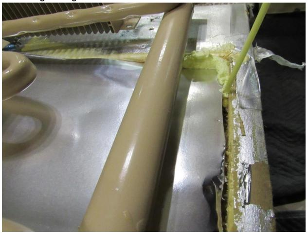
In some areas it might seem to be tight against the box, and in this area cut back enough foam on a angle to create a small gap off the unit so you can get your foam straw in to fill the void further down. We cannot stress enough on this step because if even a small 2" gap is left open it will not cool in the fridge like it should.
