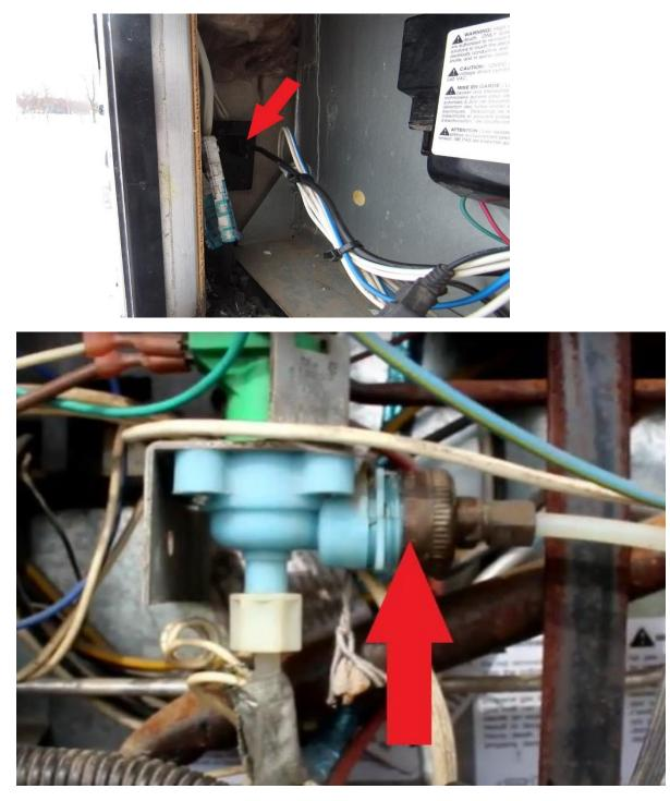
Using 2 wrenches remove the LP line (RA) off of the LP solenoid valve. Make sure LP gas is turned off.
