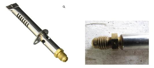
You start by taking 2 crescent wrenches and loosening the flare nut by the brass orifice, you will notice the orifice is backed away from the burner tube (above), this adjustment is done here and should stay that way, otherwise the burner will not work correctly. Do not over tighten the burner to the gas line as this might create a flare crack, yet you do want it tight enough so you do not have a gas leak.
