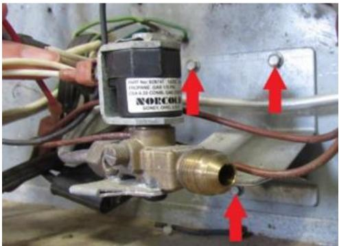
Install the three screws into the LP solenoid valve as shown.
