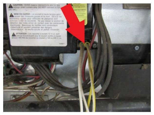
Unplug your 120v plug (RA) from your RV. Location will vary from coach to coach, if you have an icemaker unplug its cord from wall socket, making sure water pump is turned off unscrew water supply line from solenoid (RA).
