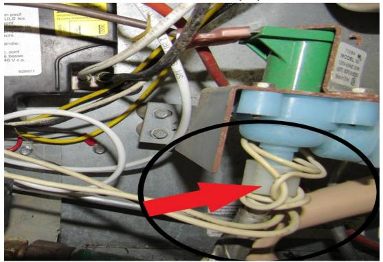
Now we need to connect the two white heater wires that run with the ice maker water hose. Connect one into the brown wire (RA).
