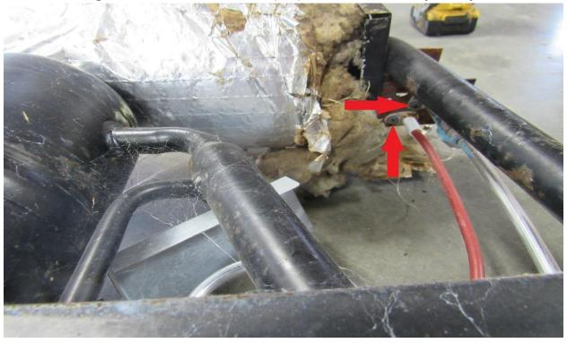
Remove the igniter and burner screws (RA). These are usually Phillips screws.
