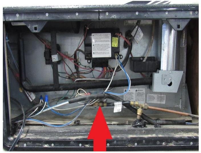
There are many different styles out there but most have at least 2 mounting screws through the back plate holding the fridge to your RV floor. Screw size and bit needed will vary from coach to coach. Remove these screws or bolts (RA).
