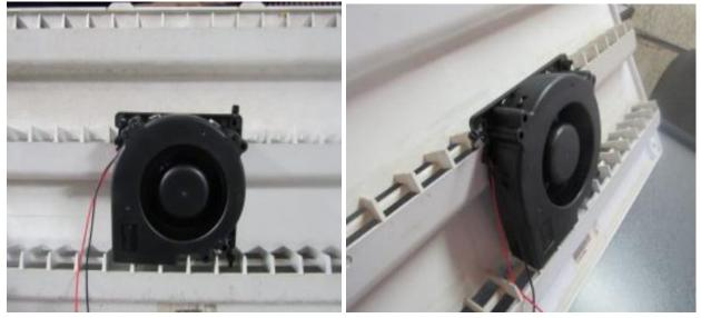
The eyelet can be screwed at any ground, connect female + to the fan switch wire, so it comes on when the lower fans come on
