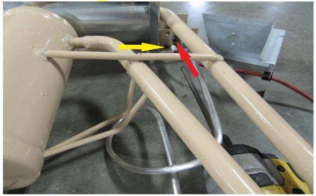
Using the original ¼" screws. Install the burner housing as shown (RA). Make sure you have approx. ¼" gap between burner tube and igniter electrode. (YA)
