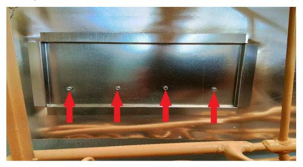
Locate your ventilation fans. Remove the 4- <sup>1</sup>/<sub>4</sub>" screws on the fan bracket (RA).
