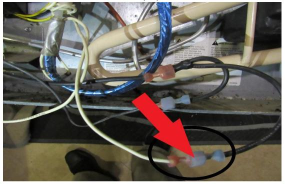
Or if everything was disconnected, this can get complicated, so you can use this as a guide to wire up your icemaker waterline heater as well, if you are not travelling in temps below 32F then this step does not have to be used. 2 brown thermostat wires blue circle.
