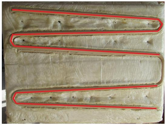
Lay unit into box being careful so as not to scrape off any thermal mastic on the box.
