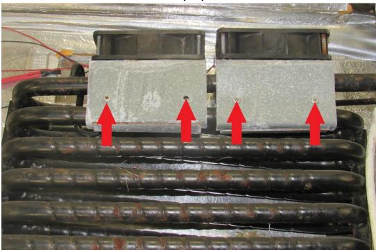
Remove the 4 fan bracket screws (RA).
