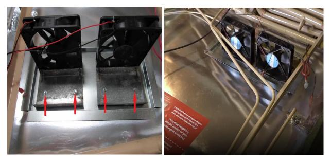
The red wire coming from the fan switch has a 3-way split. Plug the red fan wires into that as shown (RA).
