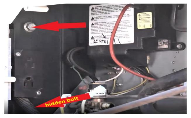
Going inside, remove all food items and start by removing the 4 black button covers on the top and bottom. (RA) Remove the 4 mounting screws on top and bottom (RA). Older style fridge trim might not have the external screw buttons but screws will still be underneath the trim after trim is removed. Screw size and bit needed will vary from coach to coach.
